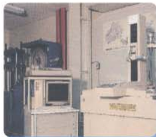
CNC Gear Tester
